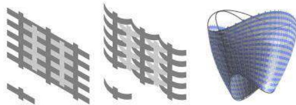
Figure 1: Lamination of two materials with different swelling coefficient that deform it specific conditions. - Prototyping a self-ventilating building skin with smart thermo-bimetals. Figure 2: Render of the intelligent skin.
