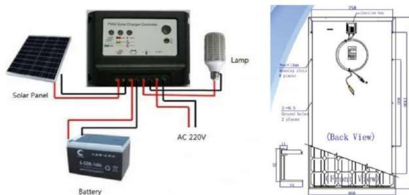
Figure 2 Principle of solar street light function and front/back views of the panel
