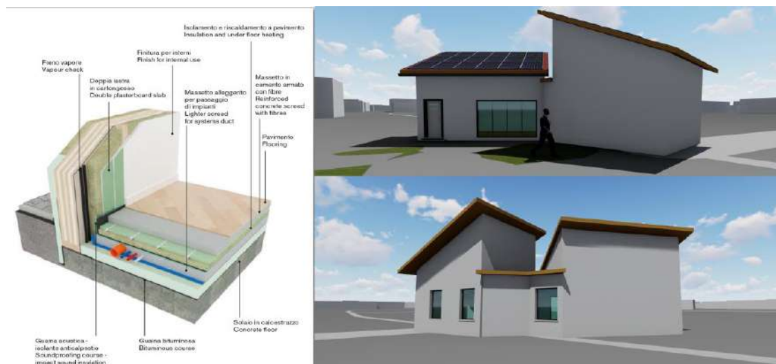
Figure 2: Xlam DolomitiProduction technological section: example of wall-raft foundation stratigraphy and render views.
